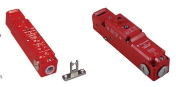
A 24V DC enhanced version is available with diagnostic output, which may be used by a control system to indicate whether a guard door is open or shut independently of the lock mechanism status. A built in LED further visually indicates the status of the switch as "door open," "door shut and unlocked," and "door shut and locked."
